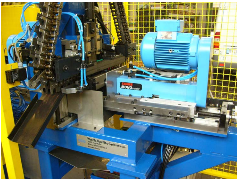
End conditioning machine (chipping) with working unit
