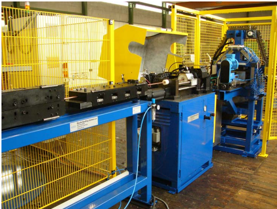
Tube cutting machine RTA 35 with straightening section - supply via coil - as well as interlinked with end conditioning machine
