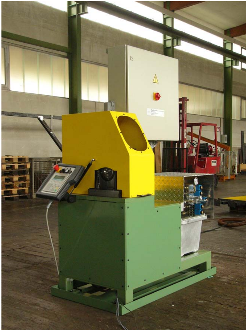
Tube cutting machine "Trennomat" - manual feed
