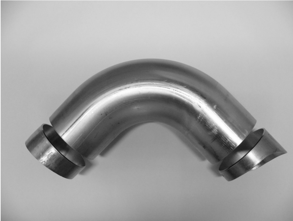
Chipless cut curved tube out of high-grade steel, Ø 102 mm, wall thickness 2 mm
