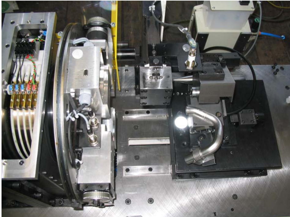
ROTAK with curved tube placed into the base part of the clamping device
