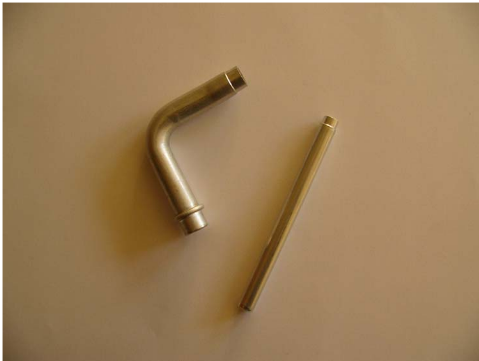
Cut curved tubes out of Al-alloys with chipless forming tube reduction (done at the same time !)
