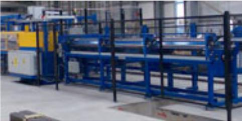
Cut tubes and pipes out of steel, stainless steel, Al- or copper alloys **chipless and with low burrs**
