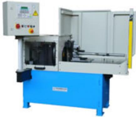
The ROTAK SR 80 is used to cut chipless surplus lengths at curved tubes and pipes. During this process the ends can be chamfered or the inner diameter be formed.
