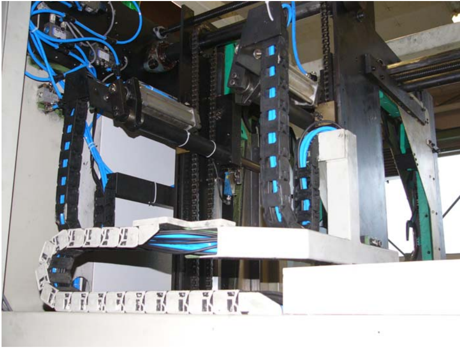
Input unit with buffer chamber and supporting arms
