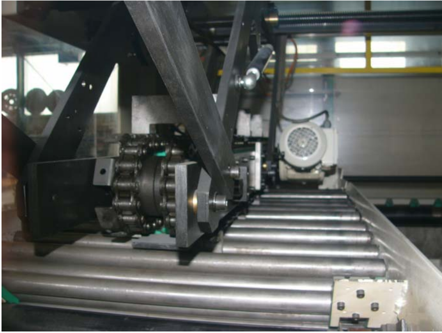
Tube / pipe conveyor at the output unit
